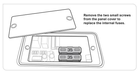
The fuses included with the Technophonic amplifier are to replace the internal fuses and only protect the amplifier itself in case of short-circuit. To replace the internal fuses, remove the panel on the bottom of the amplifier and replace the blown fuses as needed. Use only 35-amp fuses.
