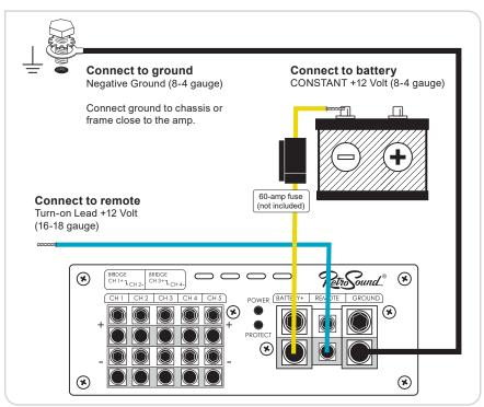
Installing a 60-amp in-line fuse near the battery on the + 12 Volt lead is required to protect your vehicles wiring and the amplifier. A high-quality barrel fuse holder and 60-amp mini-ANL fuse are available in RetroSound® Amplifier Wiring kits.
