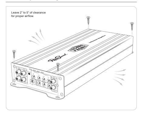
It is best to mount the amplifier in a location that allows air to freely circulate around it and allows access to the end panel controls for adjustments. Although both thermal and overload protection are built in, if the amplifier overheats it will reduce its power output to maintain operation.
