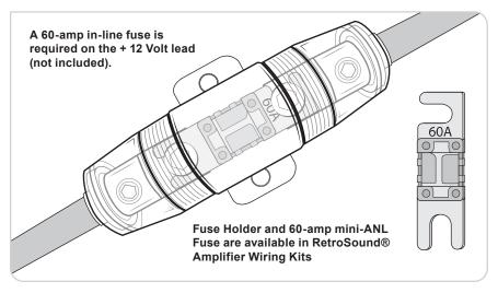
Always check the external fuse for failure first, then the internal fuses on the bottom of the amplifier. The internal fuses will only blow if the external fuse fails .
