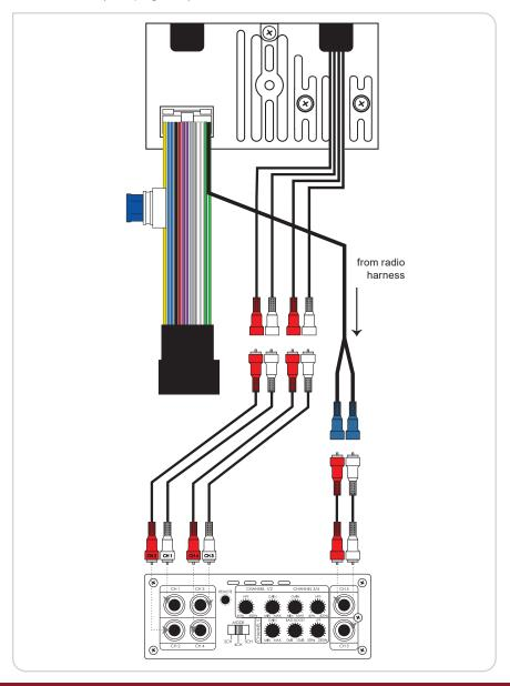
For five speaker systems, connect the speakers to channels 1-5. Strip 1/2 inch (12 mm) of insulation from the end of each wire and twist the ends. Back out the set screws 3/4 of the way out and insert each wire firmly and completely, leaving no exposed wire. Ensure each wire is inserted into the proper positive or negative terminals. Use the supplied hex wrench to tighten the set screws until snug, do not over-tighten.
