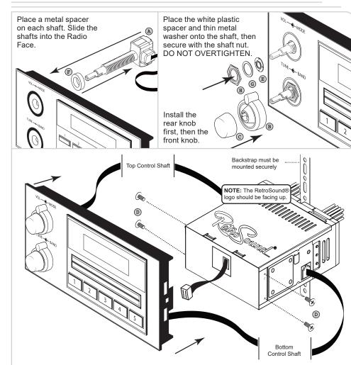
Plug the ribbon cable from the Radio Motor into the Radio Face. Attach the Radio Face to the Radio Motor with the four small screws. With the Radio facing towards you, plug the top Control Shaft into the left side of the Radio Motor. Plug the bottom Control Shaft into the right side of the Radio Motor.
