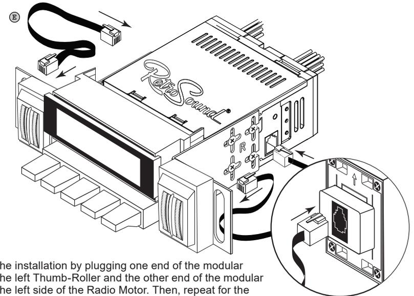
Complete the installation by plugging one end of the modular cable into the left Thumb-Roller and the other end of the modular cable into the left side of the Radio Motor. Then, repeat for the right Thumb-Roller on the right side. Use the optional hardware (if needed) to help mount the radio to the dash.
