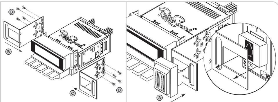
Attach each InfiMount Bracket to the Radio Motor with the eight small screws.
