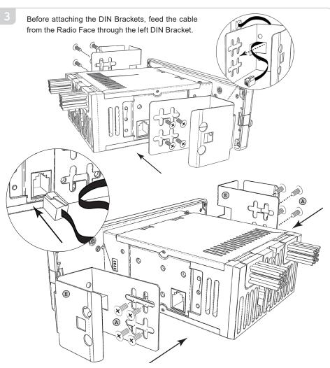
Using the 8 screws included in the Radio Motor box, install the DIN Brackets (included with the DIN Kit) to the sides of the Radio Motor. Adjust the brackets forward until they meet the back of the radio face. Be careful not to bend the brackets to ensure proper fitment into the DIN Sleeve. Plug the cable from the Radio Face into the Radio Motor.
