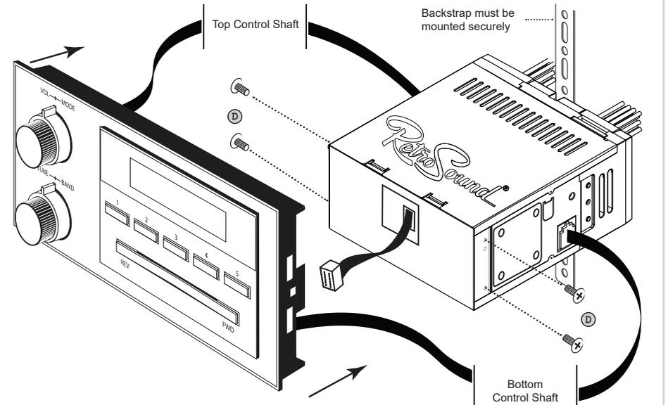
Plug the ribbon cable from the Radio Motor into the Radio Face. Attach the Radio Face to the Radio Motor with the four small screws. With the Radio facing towards you, plug the top Control Shaft into the left side of the Radio Motor. Plug the bottom Control Shaft into the right side of the Radio Motor.
