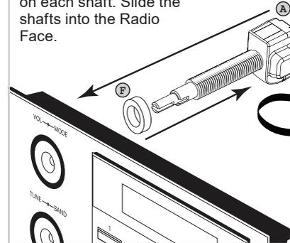
Place the white plastic spacer and thin metal washer onto the shaft, then secure with the shaft nut. DO NOT OVERTIGHTEN.
