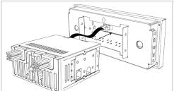
Plug the ribbon cable from the Radio Motor into the Radio Face.
