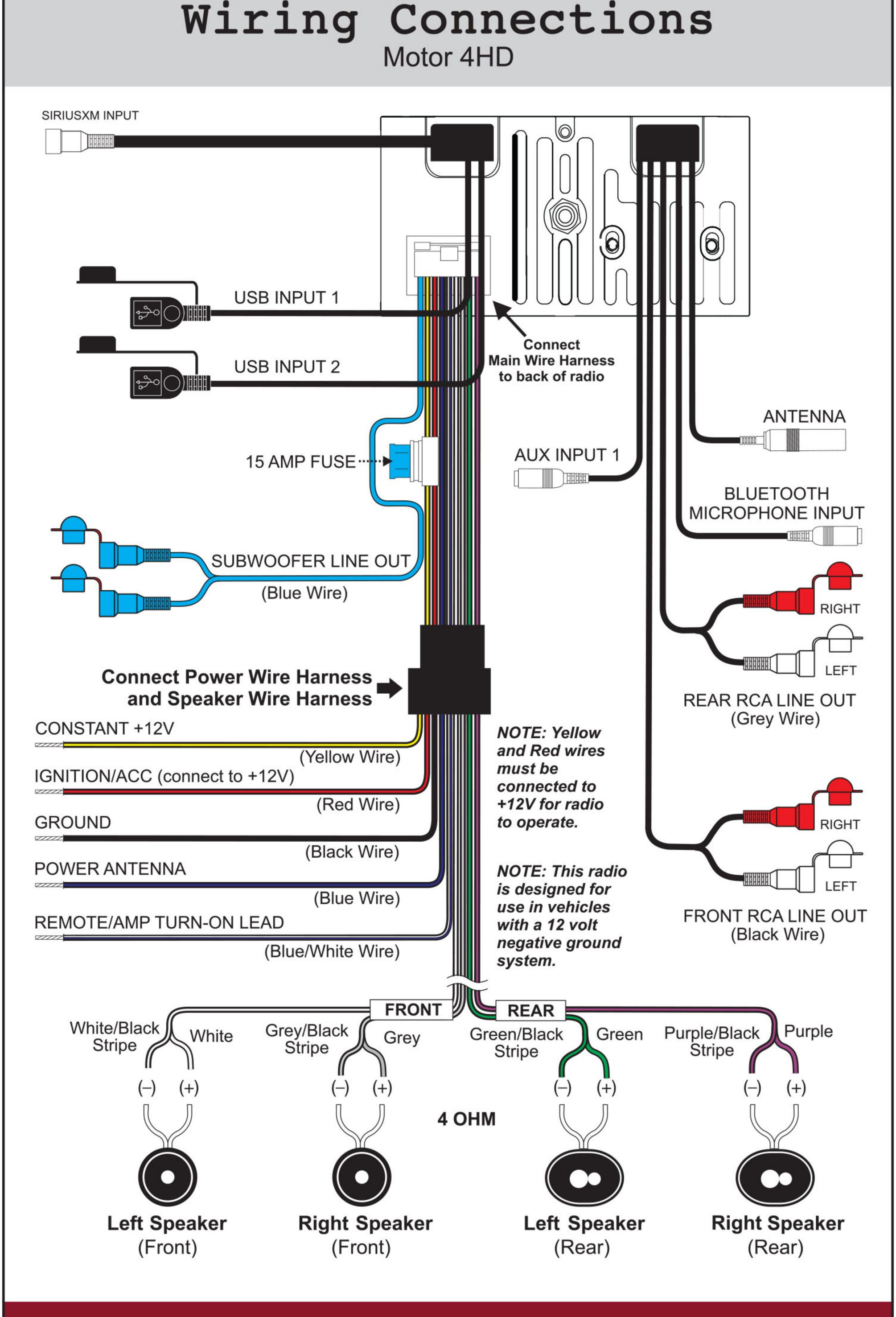
NOTE: Cutting the wiring harness, antenna lead, USB, or AUX cable will void your warranty.
