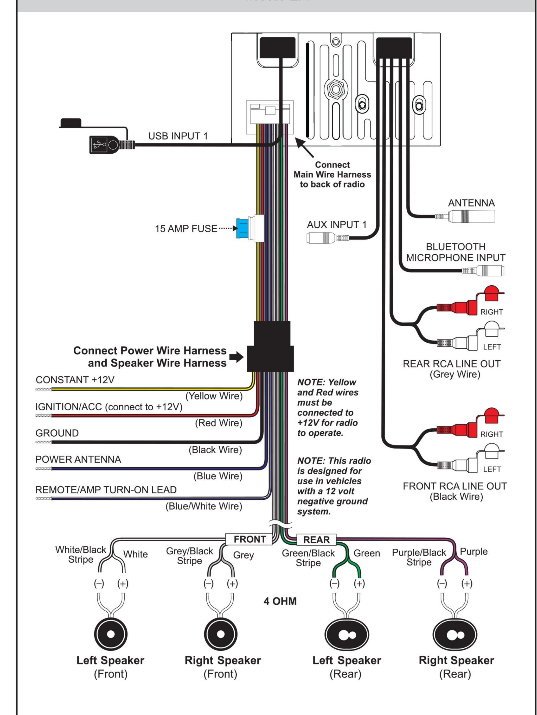
**NOTE:** Cutting the wiring harness, antenna lead, USB, or AUX cable will void your warranty.
