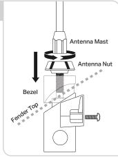
First add bezel and nut to base, then secure the antenna mast.
